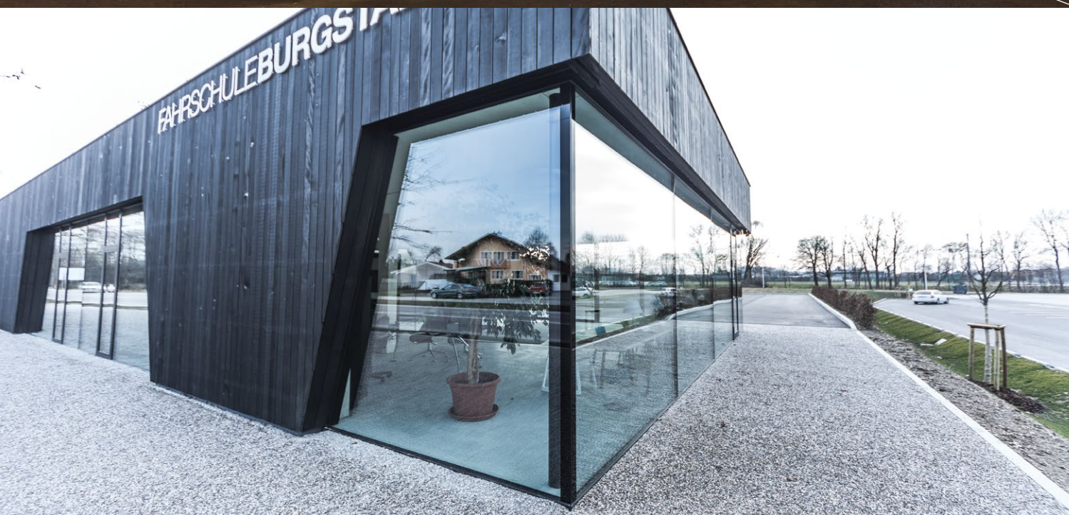
Polygonal, slanted and straight all-glass elements combined with modern facade elements
